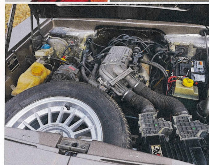
The Scimitar originally used the 3-litre Essex V6 provided by Ford, but when that became obsolete Reliant fitted the firm's Cologne unit as found in the Capri 2.8. Middlebridge used the later 2.9-litre unit from the Sierra/Granada.
