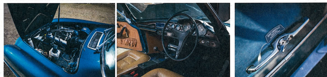
The Volvo's four-cylinder is the B20 unit from the Amazon range, equipped with Bosch's electronic D-Jetronic injection for a handy 135 bhp. The car's elegant detailing is very different from the '70s Reliant, both inside and out.
