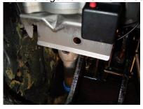
A new steering wheel boss of correct diameter may be required (from Wood and Pickett, MGF boss is the same as an early Mini).
