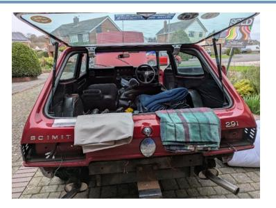
The Body was almost ready to lift off but a few small tasks remained; heater hoses, hand brake cable, gear knob and stick, fuel pipes, steering separation, various earthing points. The car was now starting
