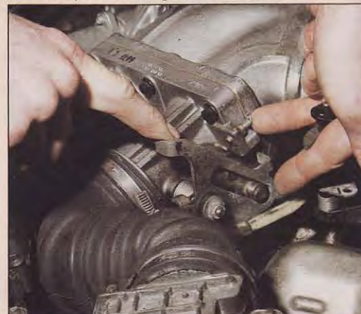
The throttle stop and roller bearing linkage are important factors when tuning this engine.
